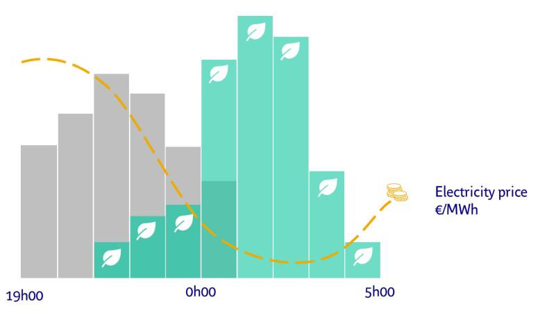
Shifting the charging of electric buses to the least expensive and carbon-intensive hours without impacting depot operations
