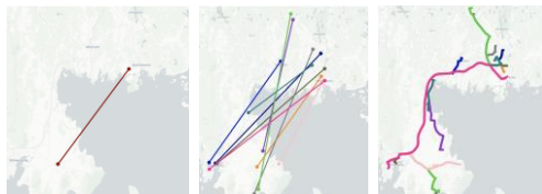
Sampling of route variants for a pair of municipalities, followed by routing along the road network
