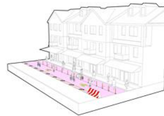
Emergency cycle track and expanded curb: Both measures help safely retain the vitality of dense areas
