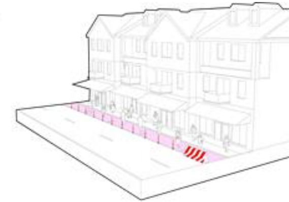
Expanded curb: parking/traffic lane re-purposed as pedestrian space to provide physical spacing
