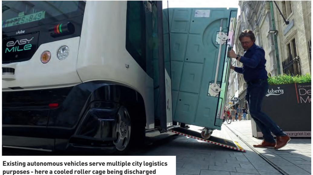
Existing autonomous vehicles serve multiple city logistics purposes - here a cooled roller cage being discharged
