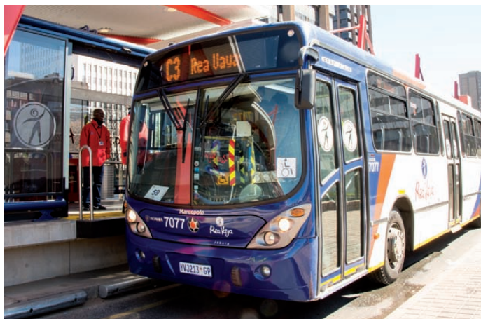
Rea Vaya BRT bus at station, showing the level entrance from the station directly into the bus
