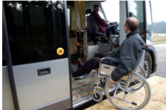
Picture 1: Easy accessible due to exact docking, wide entrance doors and level floor
