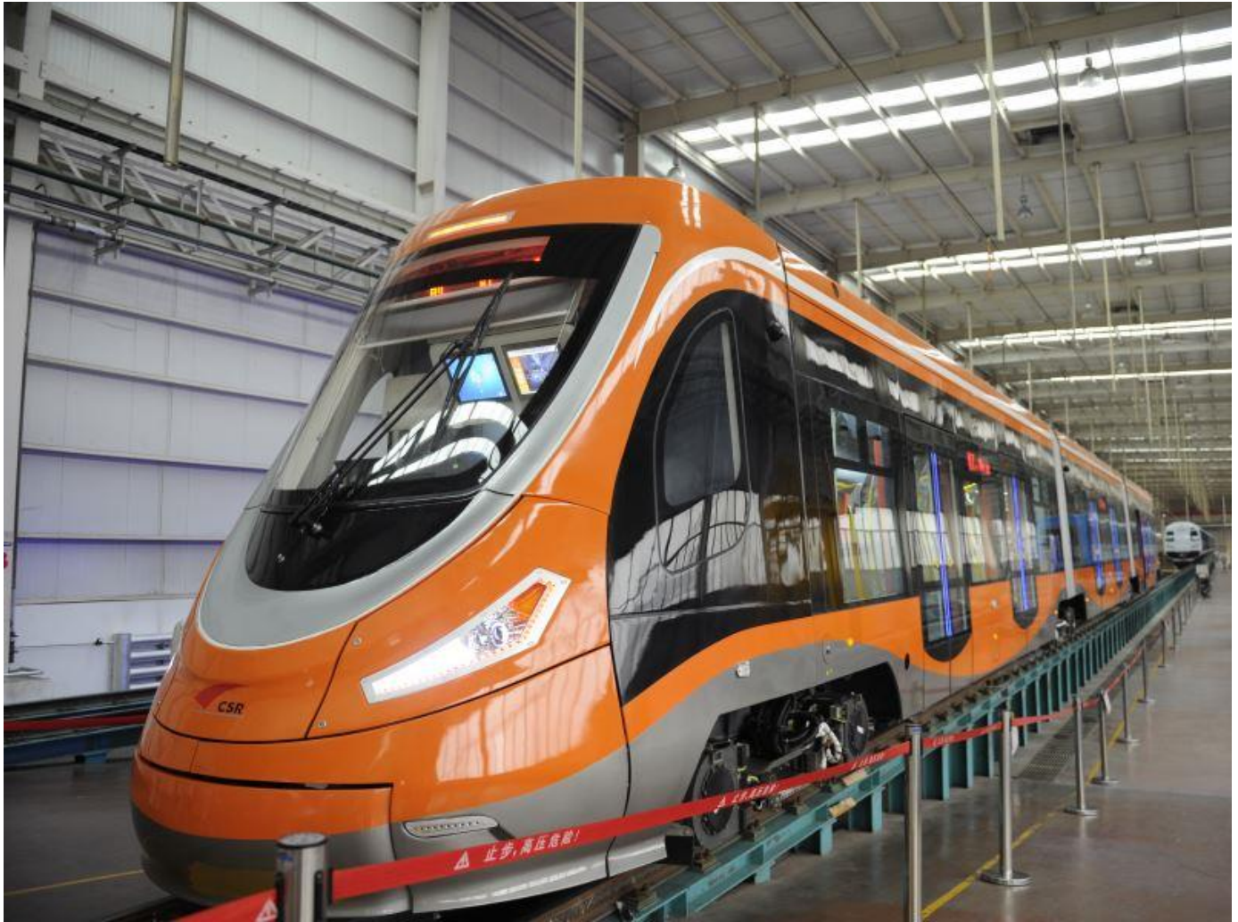
Above: Hydrail hydrogen fuel cell tram unveiled by CSR in China.
