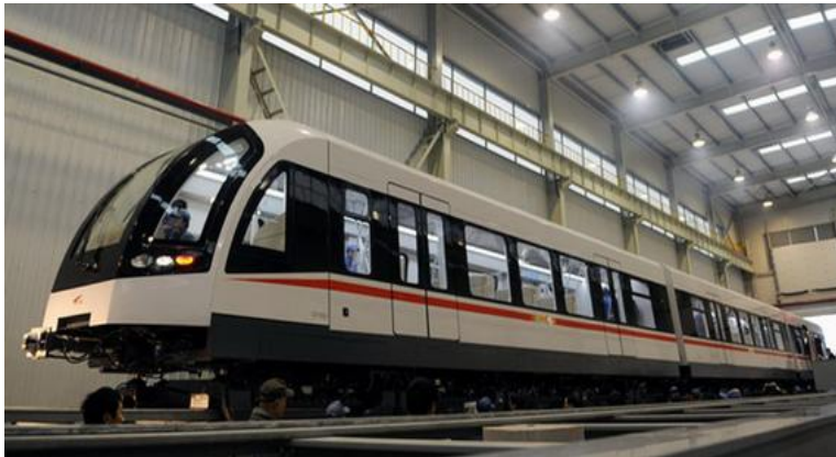
Left: The Guangzhou super-capacitor tram developed in tandem with CSR. Right: Schematics of a super-capacitor module.
