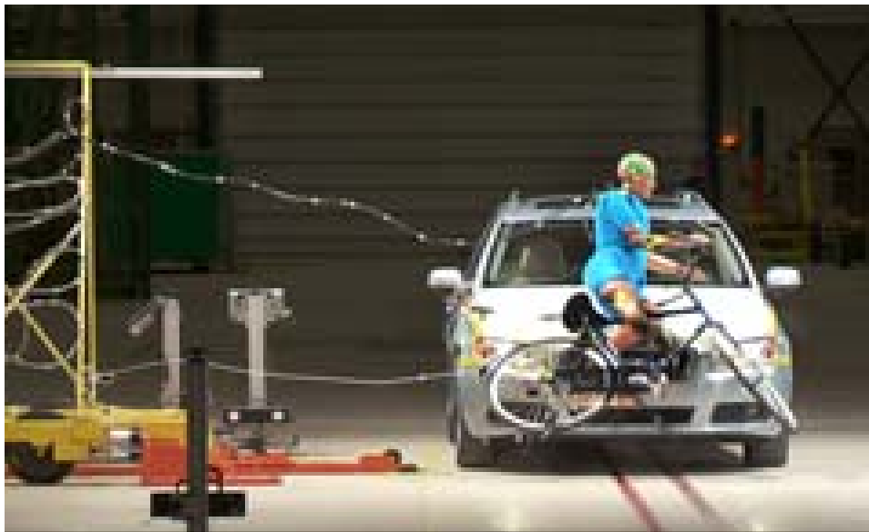
Airbag as protection of cyclists In development (TNO – APROSYS)
