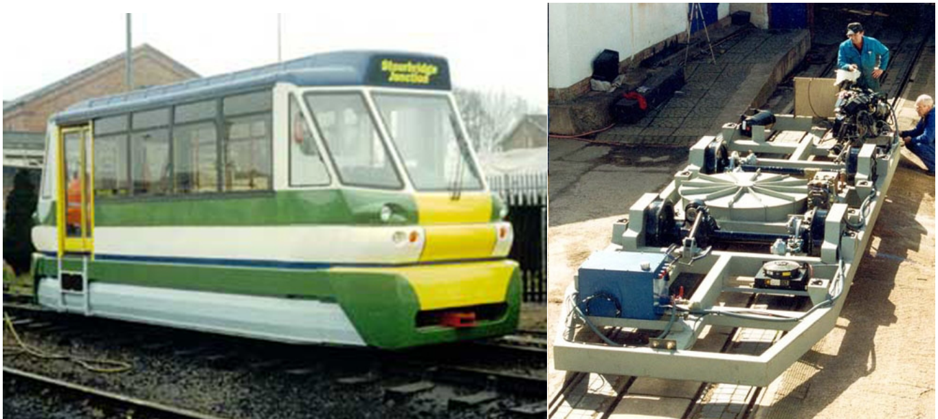
Left: A Parry People Mover tram cab running on the Stourbridge line. Right: A flywheel-enabled tram light rail chassis.
