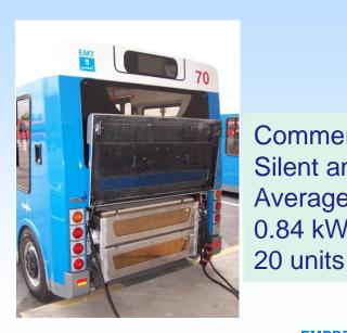
Commercial speed: 6 km/h Silent and no local emissions Average consumption: 0.84 kWh/km
