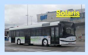
Consumption reduction: between 24 and 30 % (vs. Euro IV diesel bus)
