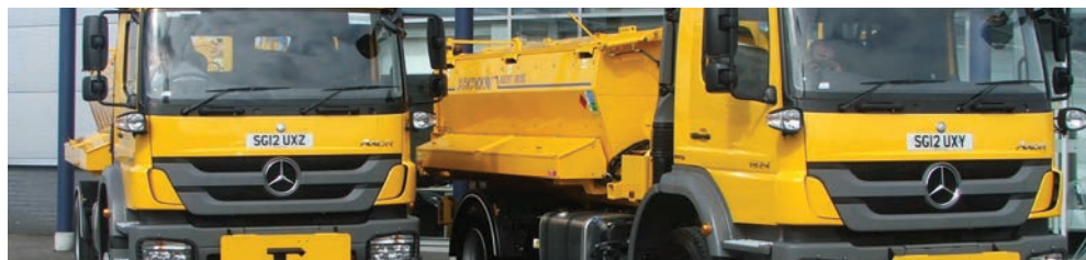
Two of Edinburgh's Council fleets newest additions: two Mercedes "hot box" trucks which are used to carry and offload hot road surface materials. (Photo: Mercedes)
