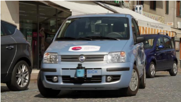
Fig. 1. Citymobil vehicle during an automatic parking manoeuvre.
