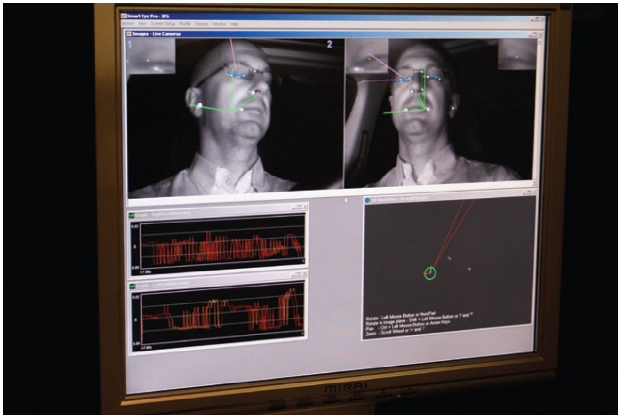
This picture shows how an eye/face tracker is used in a FOT (or other test) to collect data on driver behaviour. Source: euroFOT
