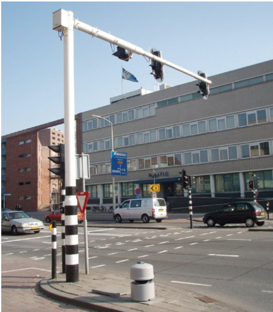
CVIS RSU next to a traffic light. The major costs for the local authority are associated with the RSUs and the control centre. Source: Peek Traffic
