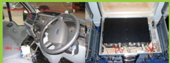
In-vehicle components & close up of CVIS OBU (a PC) used in CVIS trial in London. Source: Transport for London
