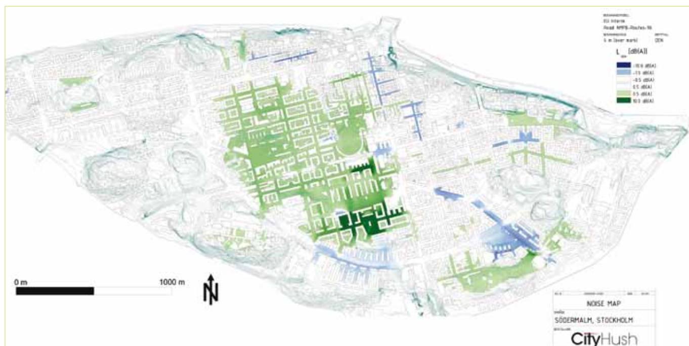
Example from an early result of a difference plot (before and after introducing the Q-Zone) for the Södermalm region in Stockholm. Positive effects within the Q-Zone are 10 – 12 dB(A)-units of noise reduction (light green-dark green colour). Some positive effects can also be seen in other areas, as well as some negative effects (light blue) just outside the Q-Zone, caused by noisy vehicles making a detour to avoid the gate-fee.
