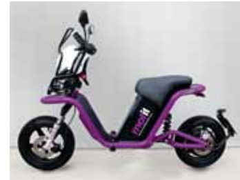
Motit electric motorbikes have an exclusive design created especially for sharing services in Barcelona. Each vehicle is equipped with a 7” screen with navigator system incorporated
