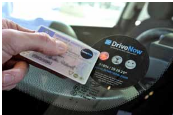
A micro-chip inserted in a sticker on your driver's licence can give you access to any DriveNow e-car sharing vehicle in Berlin
