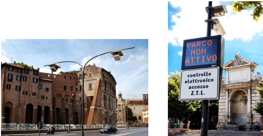
Fig 7-8 One of the first “access gates” to the city centre & the new information mini-VMS
